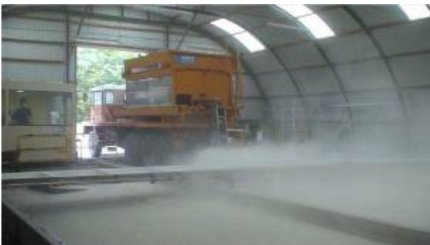
Control transverse dispersion (Cerema/Semr France)
